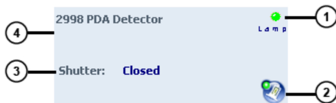
Figure 3–4: 2998 PDA detector control panel
