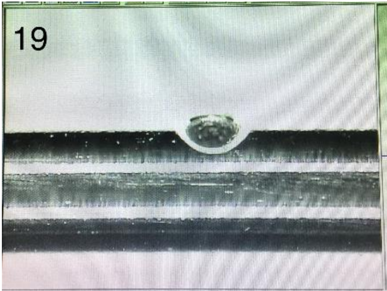
Longitudinal scratches observed
