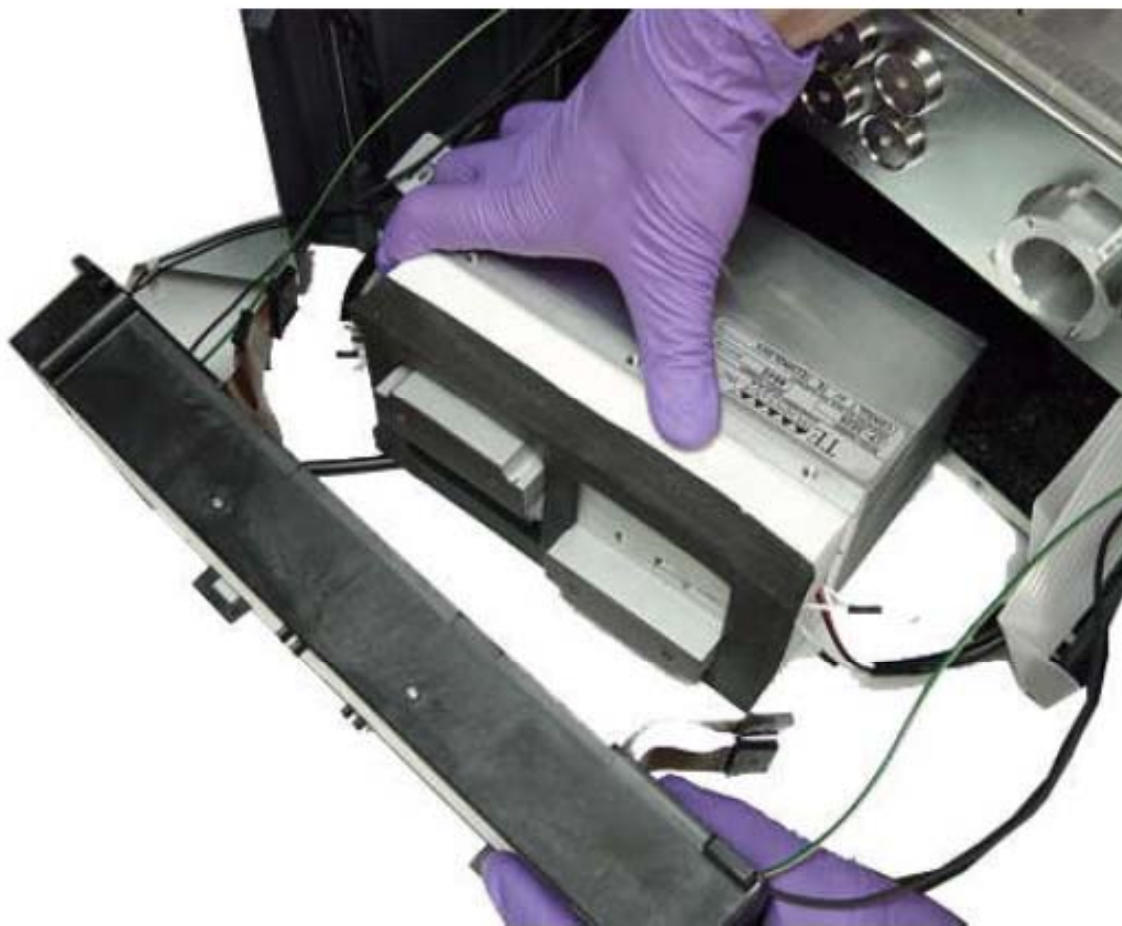
Figure 8 - Separating trough and engine assemblies
