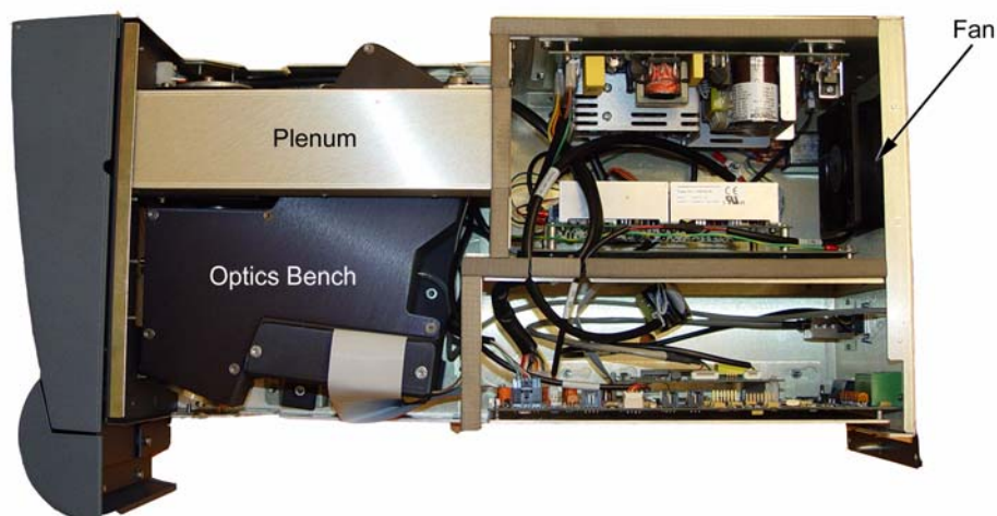
Figure 1 - Location of Fan in ACQUITY PDA
