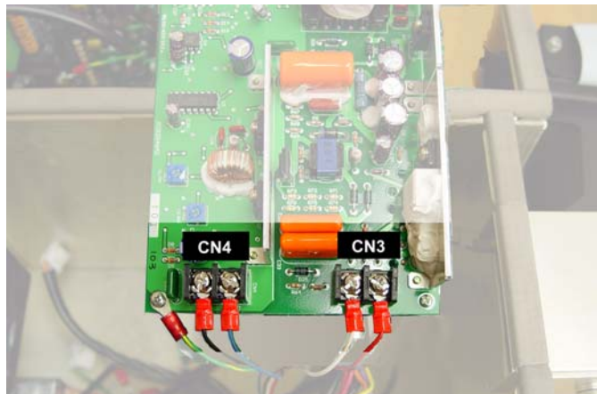
Figure 4 - Location of Lamp Power Supply Connectors
