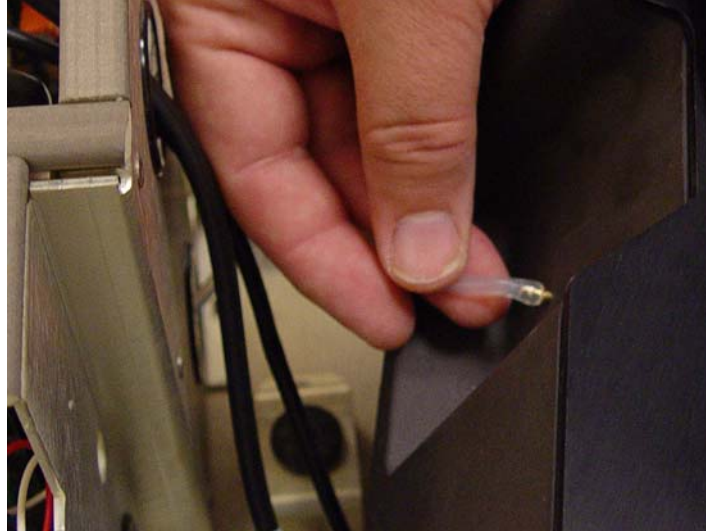
Figure 9 - Reinstalling Gas Fitting on the Optics Bench
