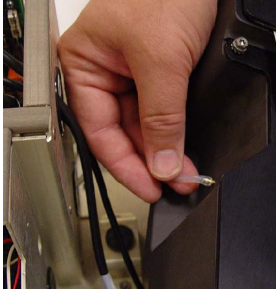
Figure 8 - Removing Gas Tubing
