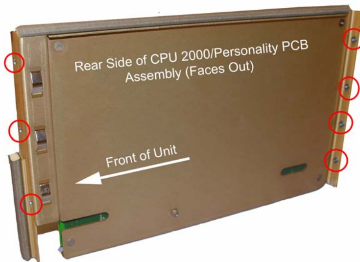
Figure 3 - Location of CPU 2000/Personality Card Bracket Assembly Screws
