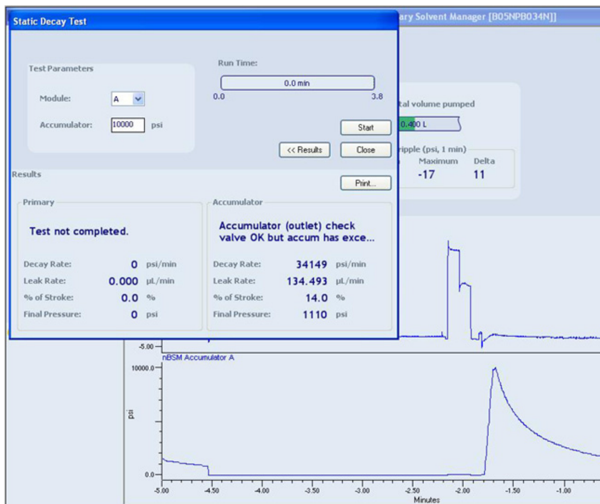
Figure 57 - Leak test (failure - primary pump)
