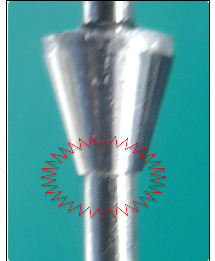
3. Outer wall collapse
