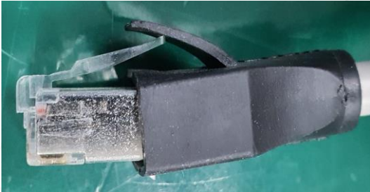
Ethernet Connector Lock – Good Condition
