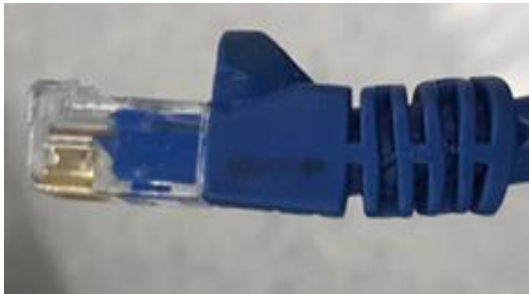
Ethernet Connector Lock – Not good Condition
