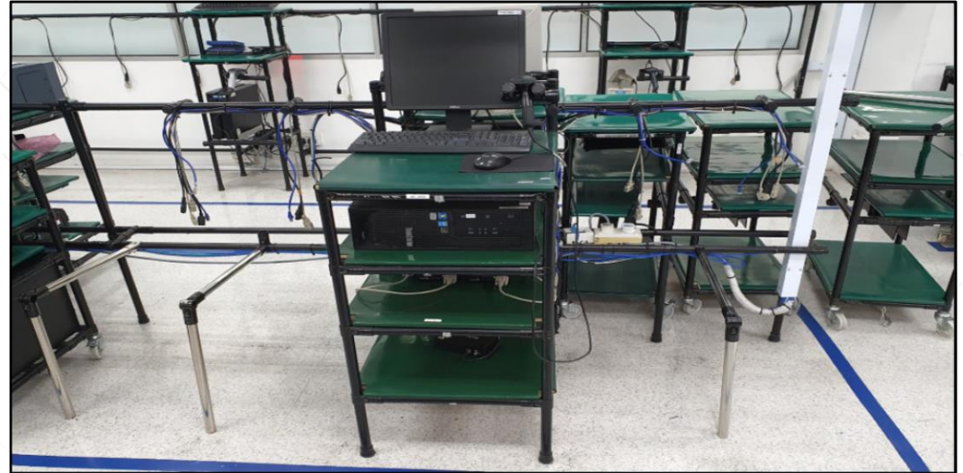
Tester with spacer in between UUT
