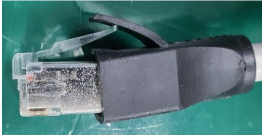
Ethernet Connector Lock – Good Condition
