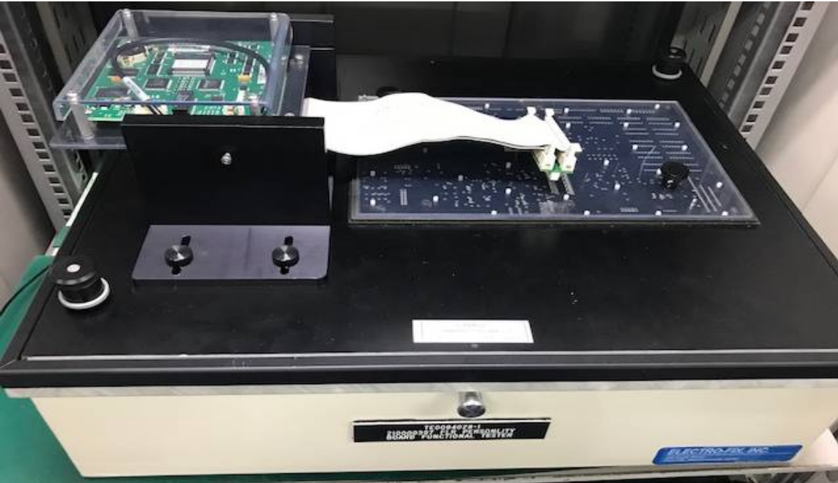
FCT Test Fixture
