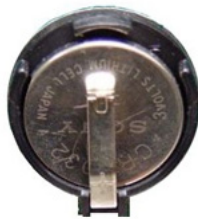
Figure 7 - 3V Lithium battery (WAT080443)
