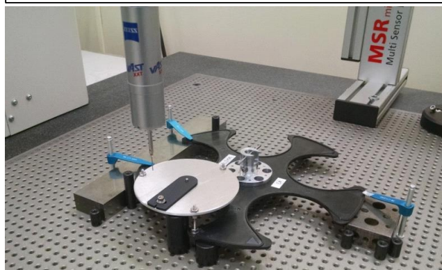
Master Carrier positioned on CMM
