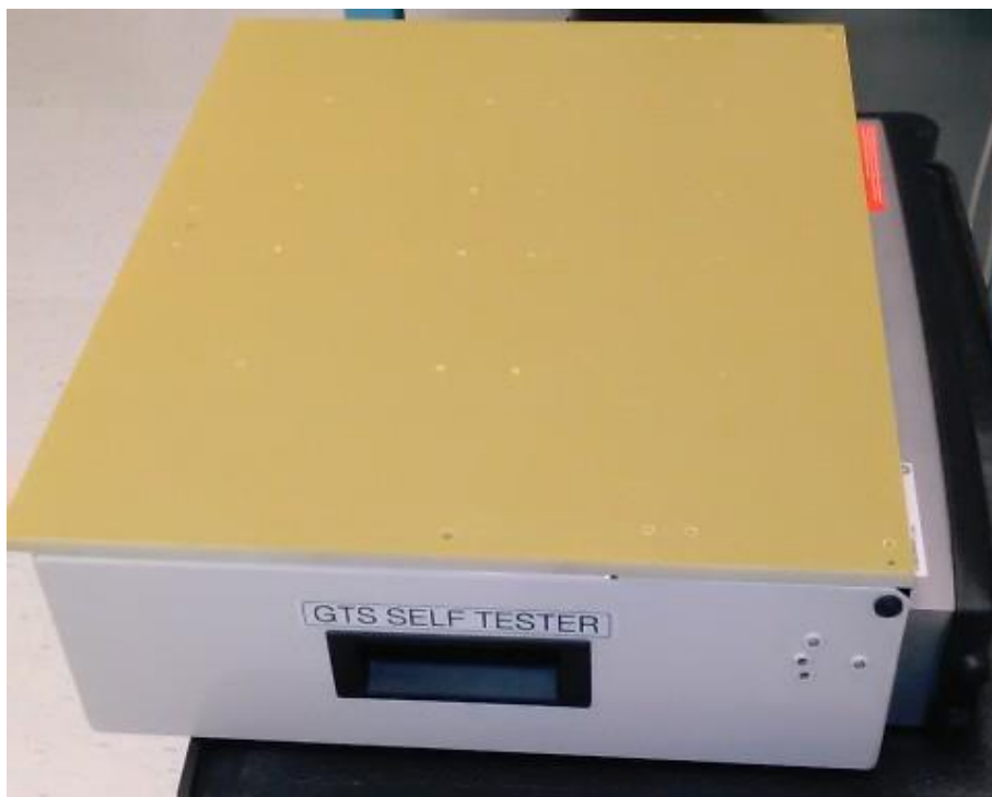
Figure 4 TE83004 GTS Self Test Fixture
