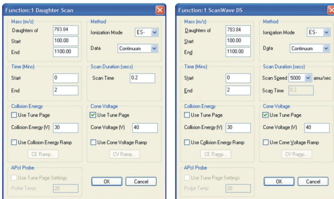
Figure 12 - Daughter scan (left) and ScanWave DS (right) parameters
