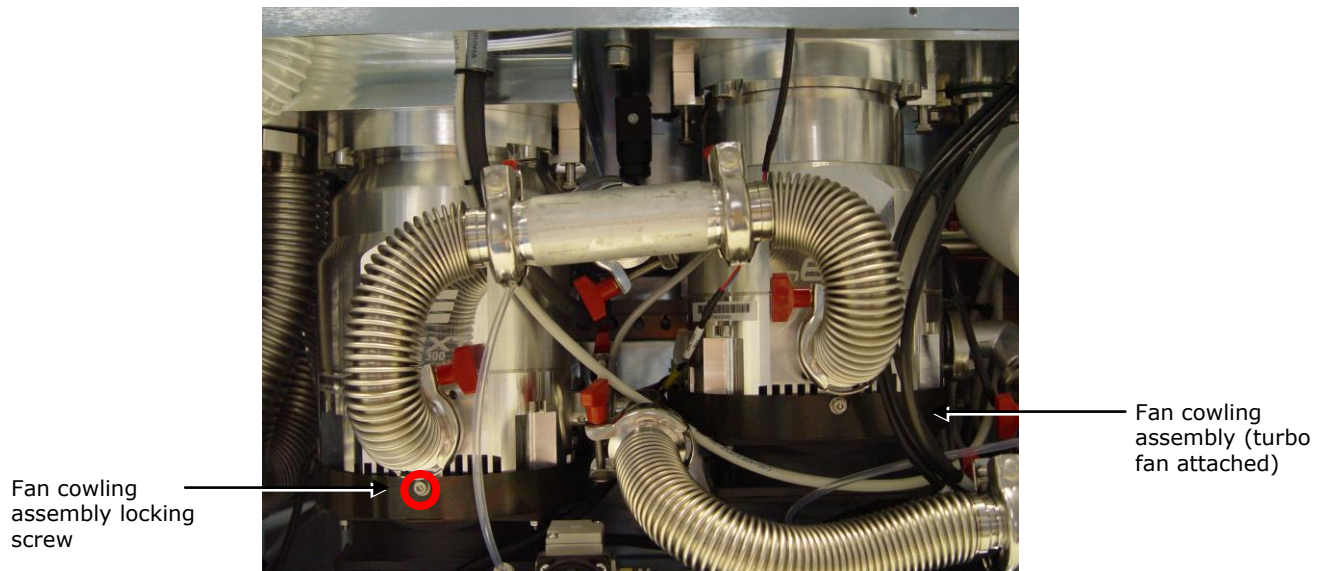
Figure 16 - Location of screws on fan cowling strip
