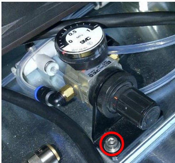
Figure 18 - Location of pressure gauge bracket screws
