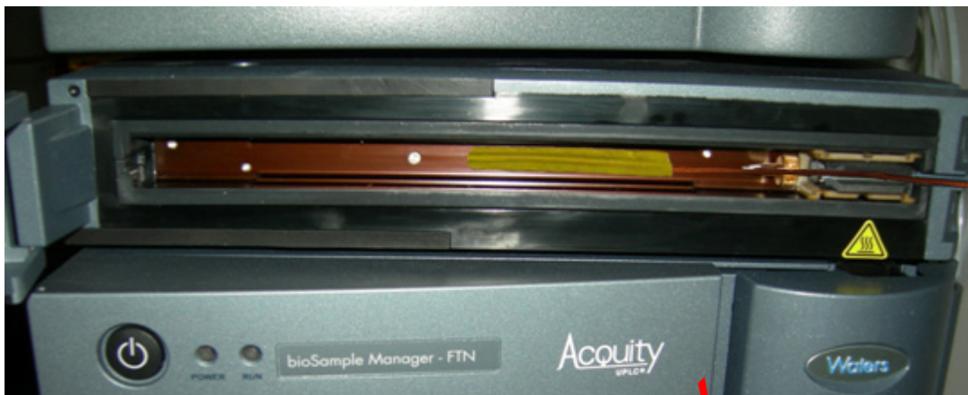
Figure 6 Routing the thermometer probe wire through the notch:
