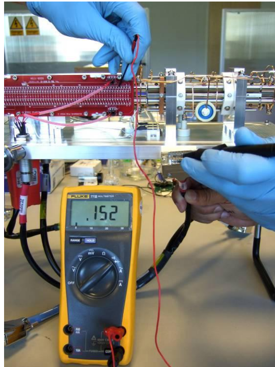
Figure 10 - Checking for continuity from D-type connector to collision cell solder points
