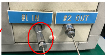
Fitting Spoiled, Replaced With Compatible One
