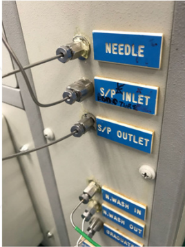
Interface Fitting & Poor Joints For Inlet/Outlet
