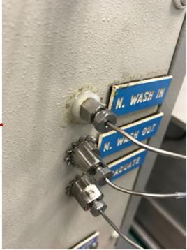
Interface Fitting & Poor Joints For Inlet/Outlet
