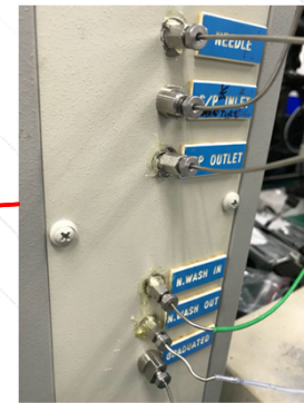
Interface Fitting & Poor Joints For Inlet/Outlet
