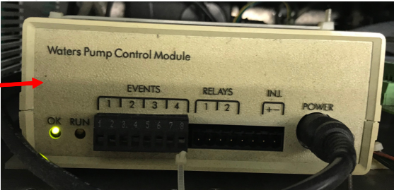
Waters Pump Control Module
