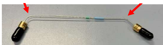
Figure 66: 0.25mm ID x 170mm MP35N Viper Capillary (P/N 6252.1924, available both as an individual item or part of capillary kit with P/N 6252.1920) connecting the Metering Device to the injection valve port 6
